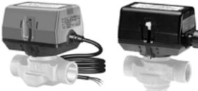
Actuator Type: Valve Fail Safe Mode: Stays in place Cable Entry: Molded strain relief, conduit clamp Dimensions, Approximate: 2.8 in. high x 3.7 in. wide x 2.7 in. deep (70 mm high x 94 mm wide x 68 mm deep) Electrical Protection: Double Insulated Ingress Protection Rating: IP40 Frequency: 50 Hz; 60 Hz Timing (seconds): Nominal Driving @ 60 Hz: 120 sec. Manual operation: Lever Mounting: Direct Coupled Shaft Adapter Type: Self-alignment Stroke: 0.4 in. (10 mm) Close-off: 60 psid
