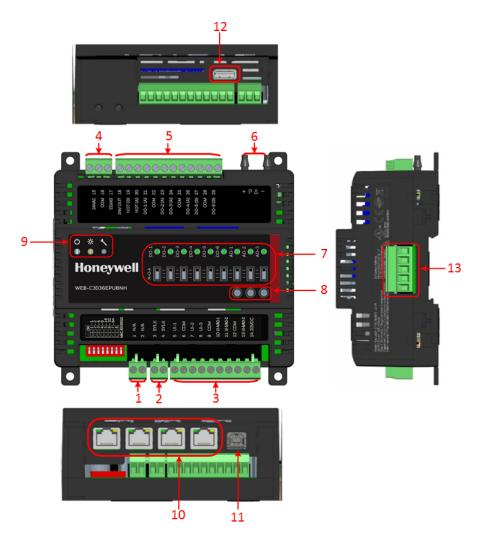
Fig. 1 CIPer 30 Controller Interfaces and Terminals
