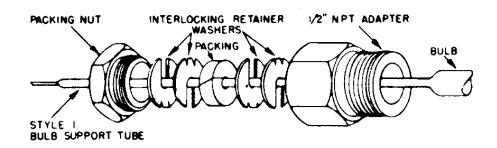
Part No. FTG13A-600R packing nut assembly. (Use with Style 1 bulb with support tube for direct immersion application.)
