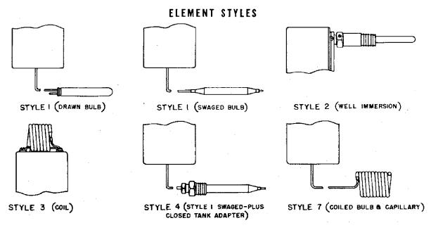
Fig. 3: Element Styles available on Series A19
