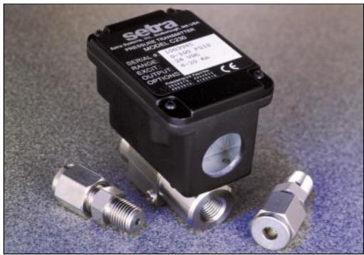
etra Systems Model 230 is a high output, low differential pressure transducer designed for wet to wet differential pressure measurements of liquids or gases. A fast-response capacitance sensor and signal conditioned electronic circuitry provide a highly accurate, linear analog output proportional to pressure. Both unidirectional and bidirectional pressure ranges are available for applications with line pressure up to 250 psig.
