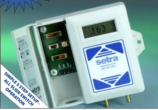
sense differential or gauge (static) pressure and convert this pressure difference to a proportional electrical output for either field selectable unidirectional or bidirectional pressure ranges. The 260 Series is offered with field selectable high level analog outputs of 1 to 5, 0 to 5, and 0 to 10 VDC, or 4 to 20 mA.
