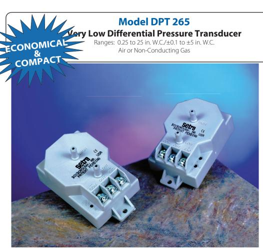
etra Systems 265 pressure transducers sense differential or gauge (static) pres-sures and convert this pressure difference to a proportional electrical output. The 265 is offered with a high level 0-5 VDC output or a 4-20 mA output. It is also offered with 0-5 or 0-10 VDC output in the 24 VAC excitation version.
