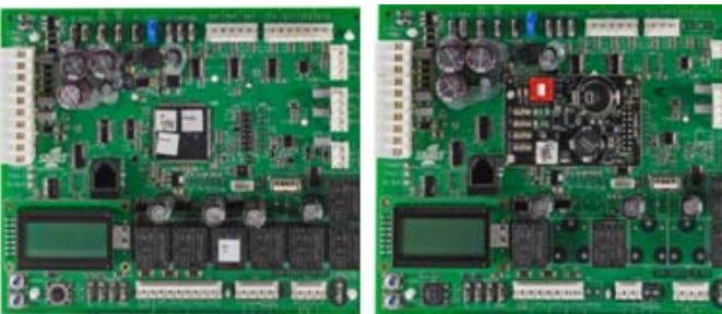
Figure 6: Unit Control Boards SE-SPU1001 and SE-SPU1002, SE-SPU1011 and SE-SPU1012
