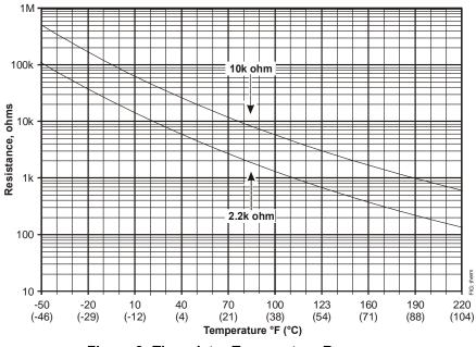
Figure 3: Thermistor Temperature Response
