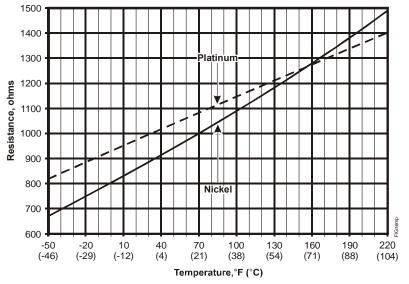
Figure 2: Nickel and Platinum Temperature Response
