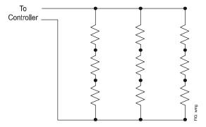
Figure 4: Nine-Sensor Series-Parallel Wiring
