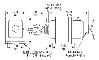
Figure 16: Dimensions for Y64T15 Type, in./mm
