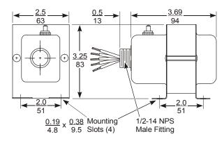
Figure 14: Dimensions for Y66F12 Type, in./mm
