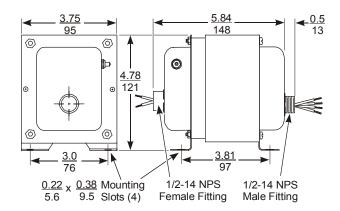
Figure 19: Dimensions for Y69T15 Type, in./mm
