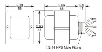
Figure 8: Dimensions for Y65F42 Type, in./mm
