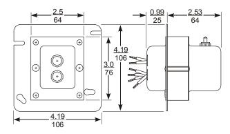
Figure 9: Dimensions for Y63T22 Type, in./mm
