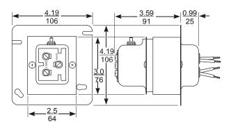
Figure 17: Dimensions for Y64T21 Type, in./mm
