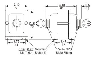
Figure 7: Dimensions for Y65F13 and Y65S13 Types, in./mm
