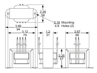
Figure 6: Dimensions for Y65T54 Type, in./mm
