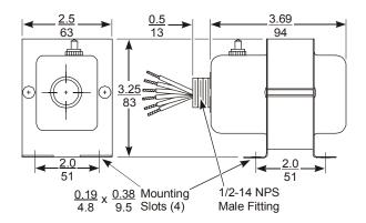
Figure 12: Dimensions for Y66T12 Type, in./mm
