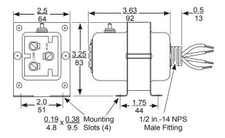
Figure 10: Dimensions for Y63T31 Type, in./mm
