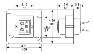
Figure 3: Dimensions for Y65A21 Type, in./mm
