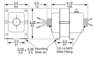
Figure 15: Dimensions for Y66F13 Type, in./mm
