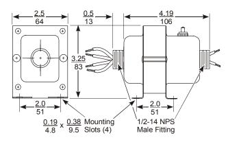
Figure 13: Dimensions for Y66T13 Type, in./mm
