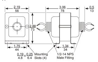
Figure 2: Dimensions for Y65A13 and Y65G13 Types, in./mm
