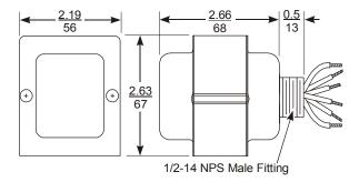
Figure 5: Dimensions for Y65T42 Type, in./mm
