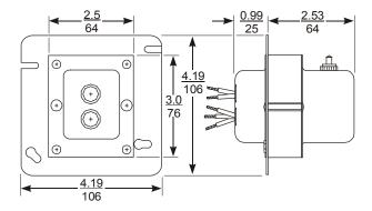
Figure 11: Dimensions for Y63F22 Type, in./mm
