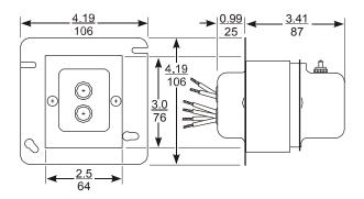
Figure 18: Dimensions for Y64T22 Type, in./mm
