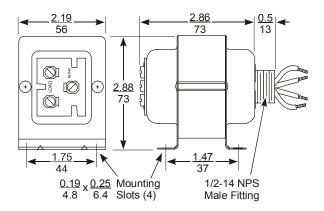
Figure 4: Dimensions for Y65T31 Type, in./mm
