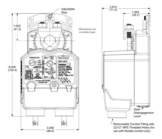
NOTE: The two holes at the top of the actuator are NOT for use in direct-coupled applications. (They are for remote mounting, such as with the optional HLO-4001 Crank Arm Kit.) For mounting to valves, see the appropriate valve installation guide.
