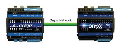
**Note:** Add to a JENE-EG534, up to 8 additional Onyxx-XM34IO extender modules (at 34 points of IO each) for a maximum of 306 points.
