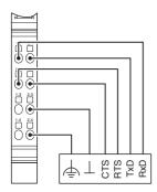
Figure 5 RS-232 interface wiring: four-wire handshake
