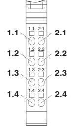
Figure 3 Terminal point assignment
