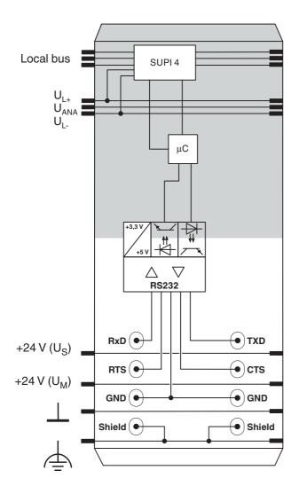
Figure 1 Internal wiring of the terminal points
