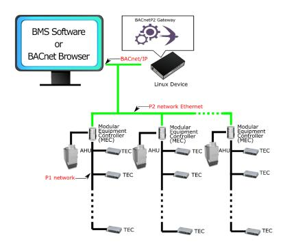
This setup is showing a P2/Ethernet connection
