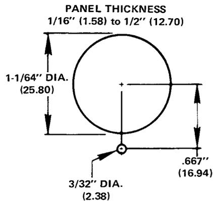
Figure-1 Minimum Centerline Spacing for Panel Cutout 2" (50.8).
