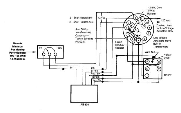
Figure-6 Solid State Paralleling Relay Used with TP-307 Bulb Microtherm for Remote Minimum Positioning.
