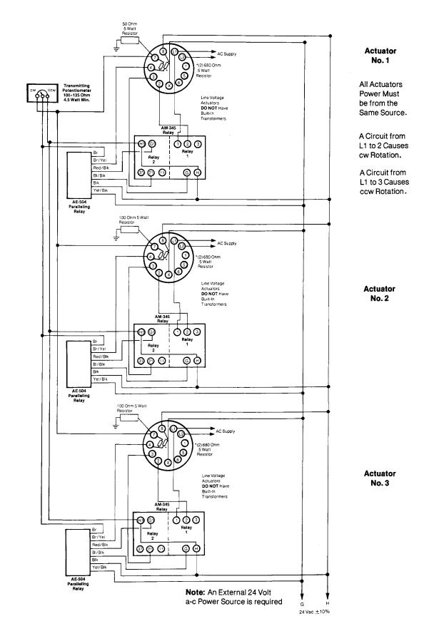
Figure-7 Solid State Paralleling Relay Line Voltage Proportional M-9200, 9400, 9600, 9800 Series Actuators (Max. 3) Positioned from Potentiometer.
