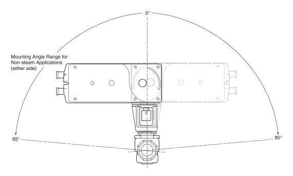
Figure-15 Typical Mounting Position.
