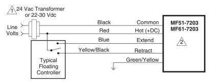
1\Provide overload protection and disconnect as required.
