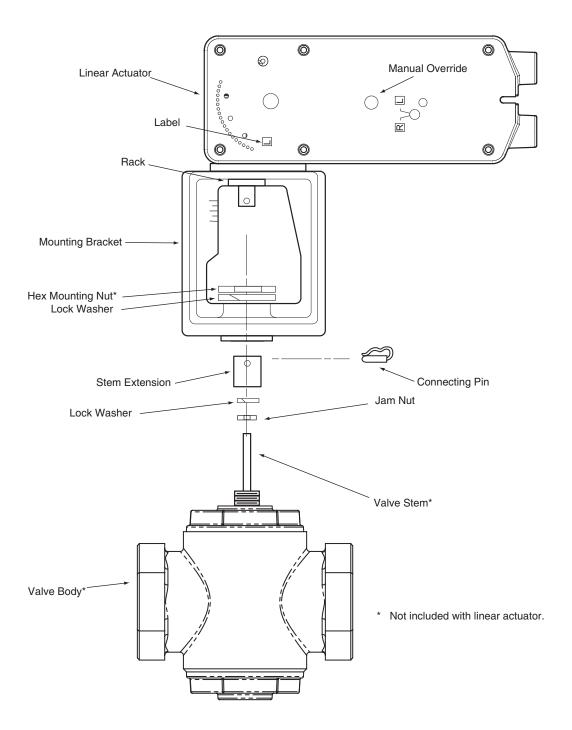
Figure-12 Mx61-720x Series Actuator Exploded View.
