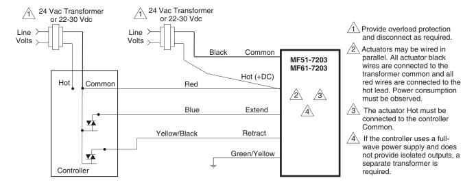
Figure-5 Triac Sink With Separate Transformers.
