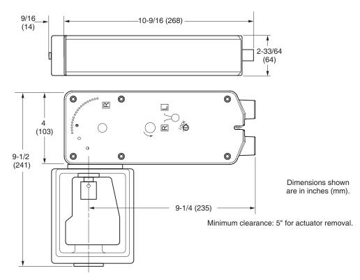
Figure-20 Mx61-720x Spring Return Valve Actuator Dimensions.
