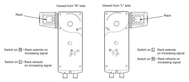
Figure-9 Rotation Switch Settings for MSx1-7203 Proportional Actuators.
