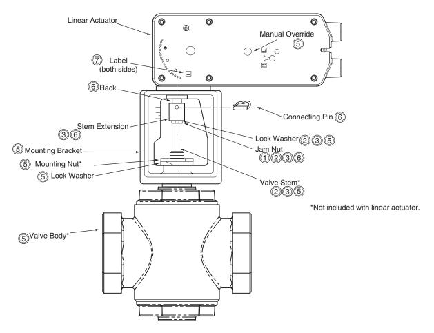
Figure-13 Typical Assembly and Installation.
