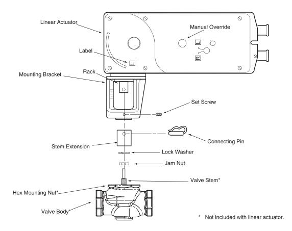
Figure-10 Mx51-720x Series Actuator Exploded View.
