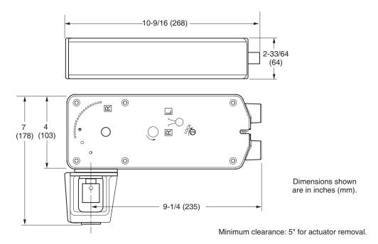
Figure-19 Mx51-720x Spring Return Valve Actuator Dimensions.
