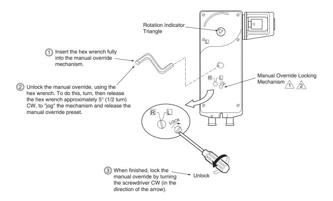
1 When necessary, the manual override mechanism may be used to reposition the actuator at any point between -5° and 85°. This mechanism is accessible on both sides of the actuator and can be used to ensure tight close-offs for valves.
