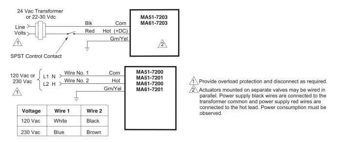
Figure-1 Typical Wiring Diagrams for Two Position Actuators.
