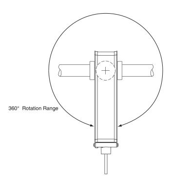
Figure-17 Actuator Positioned Anywhere Within 360 Degrees.
