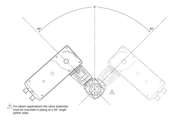
Figure-16 Typical Mounting Position for Steam Applications.
