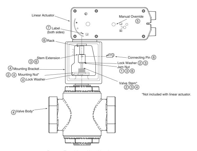
Figure-14 Typical Assembly and Installation.
