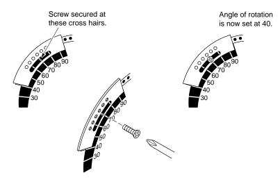
Figure-6 Securing the AM-689 Rotation Limiter.
