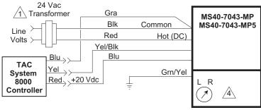
Figure-1 Proportional Control of TAC System 8000 Room Temperature Controller Application of MS40-7043-XXX Actuator.
