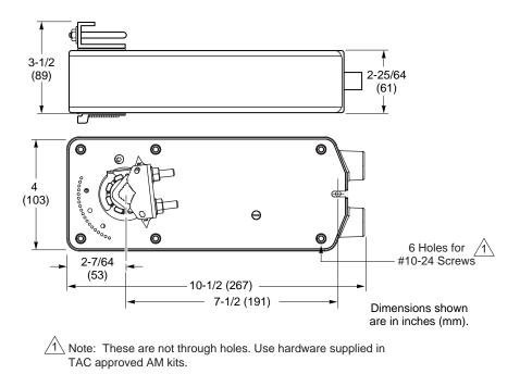
Figure-10 MS4X-7073 and MS4X-7153 Spring Return Damper Actuator Dimensions.
