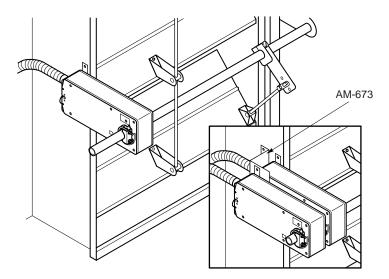
Figure-4 Mounting Multiple Actuators.
