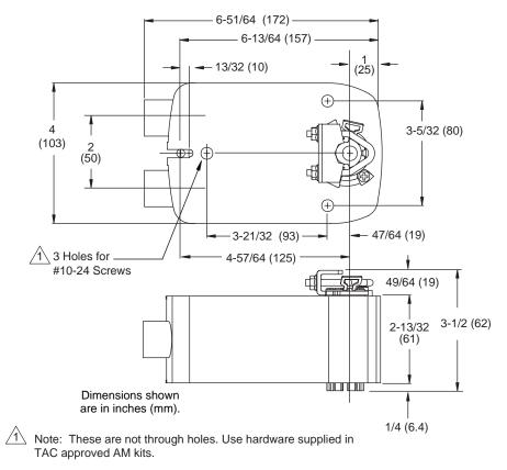
Figure-9 MS40-7043 Spring Return Damper Actuator Dimensions.
