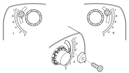
Figure-5 Adjusting Stop Block for Limited Rotation.
