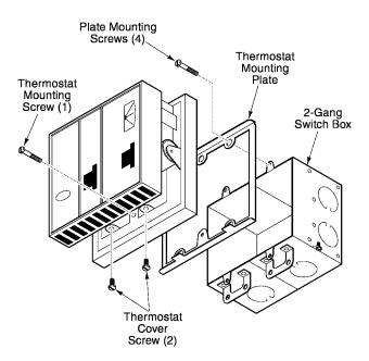
Figure-2 Thermostat Mounting.
