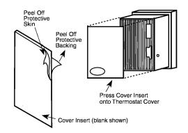
Figure-5 Cover Insert Installation.
