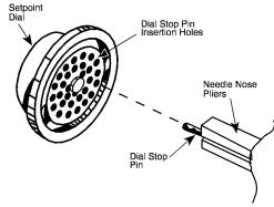
Figure-6 Dial Stop Pin Insertion.
