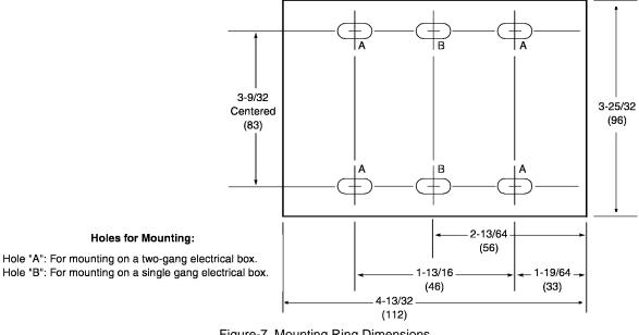
Figure-7 Mounting Ring Dimensions.
