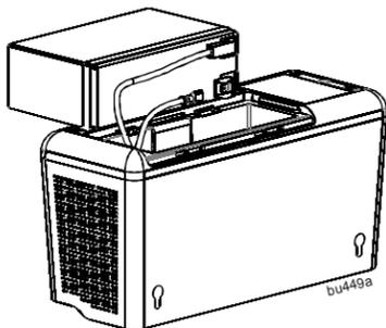
**3** Connect the battery cable securely to the battery terminal. It is normal for small sparks to be seen when the battery cable is connected to the battery terminal.
