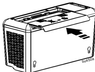
**4** Reinstall the battery compartment cover. Be sure that the release tabs lock into place.
