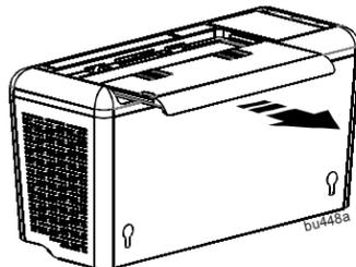
**2** Press the battery compartment cover release tabs located on the underside of the unit. Slide the battery cover off.
