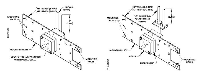
Figure 2. In Plaster Walls Use Wall Box Kits No. 192-478, 192-498, 192-480, or 192-499.
