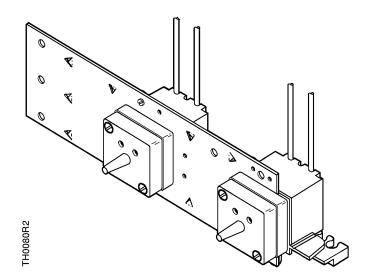
Figure 9. Terminal for Two Vertical Thermostats.
