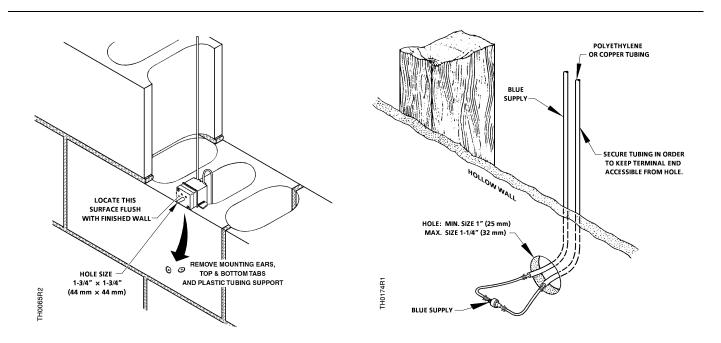
Figure 3. In Block Walls Use Wall Box Kit No. 192-478, 192-498, 192-480, or 192-499 After Removing the Mounting Plate.
