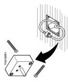
2. Pull out the terminal tubing. The terminal tubing has a supply (blue) and a return plug-in adapter connected with an air link. This provides a pressure-tight connection between supply and return for testing air lines for leakage.
