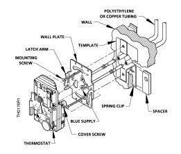
Figure 6. Mounting Wall Plate and Thermostat with Kit Nos. 192-481 and 192-685.
