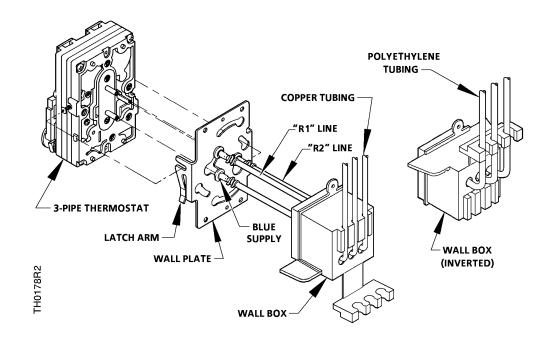
Figure 8. Installing "DNV" Thermostat Using No. 192-498 or 192-499 Wall Box Terminal.
