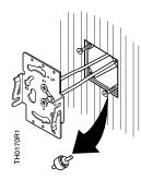
3. Remove the air link and install plug-in adapters on the wall plate.
