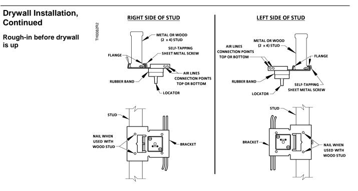
Figure 11. Drywall Mounting Bracket Positions.
