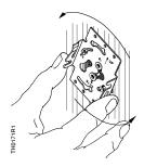
4. Install the wall plate on the wall box using the screws furnished with the instrument. Note that the wall plate has key slotted holes to allow insertion of the screws prior to installation of the wall plate and also to allow leveling of the wall plate.
