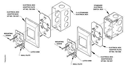
**NOTE:** Adapter frame, Part Number 192-308, may be used in conjunction with the adapter base to cover up oversized holes, paint lines, broken walls, spots etc.
