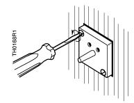
1. After the wall is finished, remove the locator using a screwdriver to remove the two screws and lightly rock the locator while pulling to free it from the plaster.
