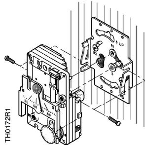
5. Carefully plug the thermostat into the wall plate.
