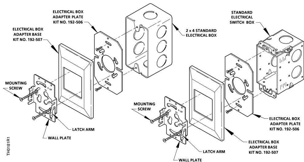
**NOTE:** Adapter frame, Part Number 192-308, may be used in conjunction with the adapter base to cover up oversized holes, paint lines, broken walls, spots etc.
