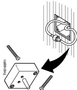
2. Pull out the terminal tubing. The terminal tubing has a supply (blue) and a return plug-in adapter connected with an air link. This provides a pressure-tight connection between supply and return for testing air lines for leakage.
