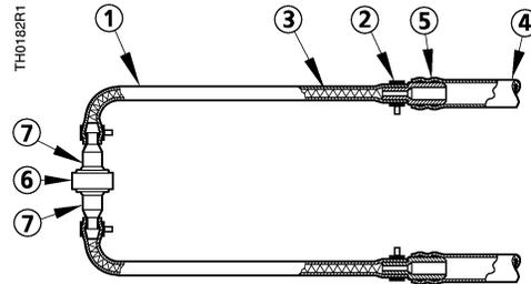
**Figure 15. Tubing Kit No. 192-481 (10/Kit) and 192-505 (10/Kit).**
