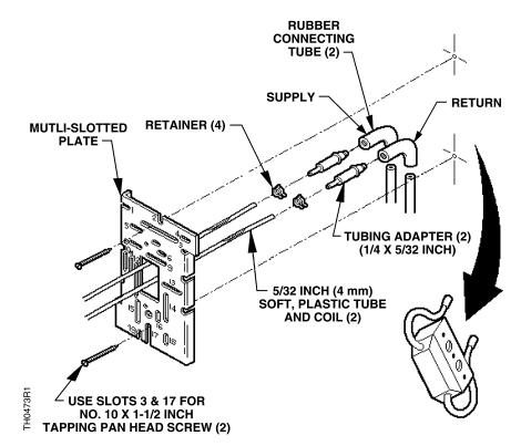
**NOTE:** Adapter Base and Plug-in Adapter (2) not shown. See *Figure 1* for proper installation.
