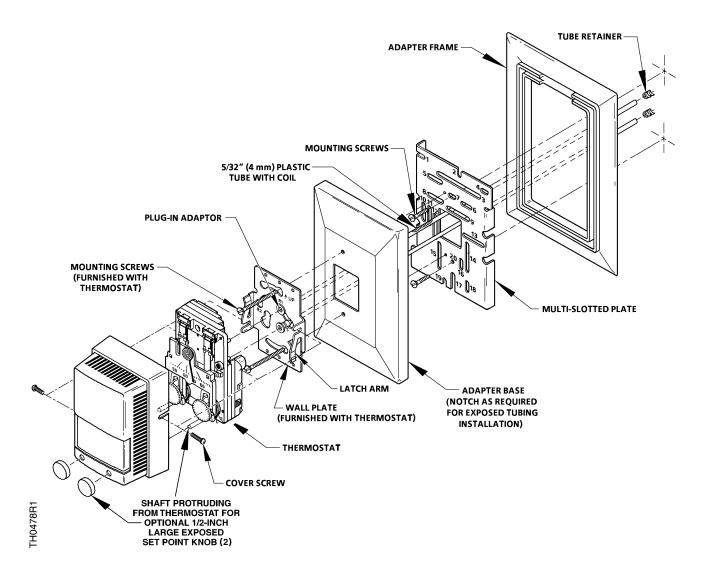
Figure 1. Typical Thermostat Installation.
