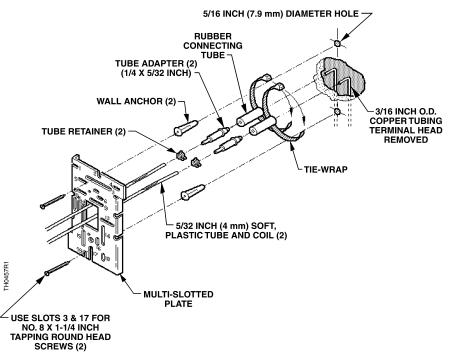
Figure 6. Terminal Head Removed with 3/16-inch O.D. Copper Tubing.
