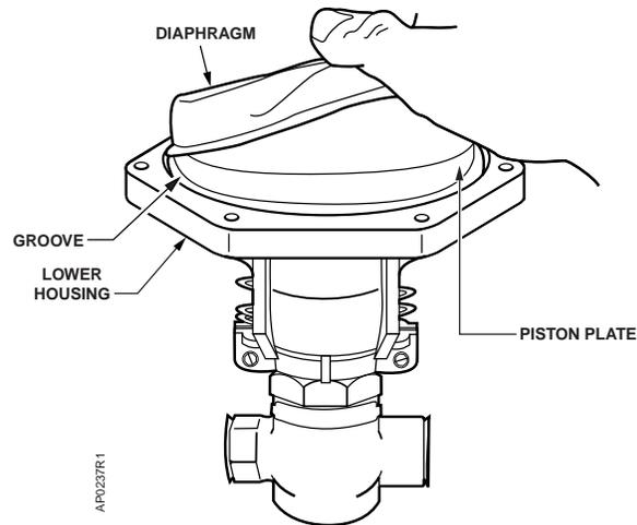
**Figure 6. Replacing the Diaphragm on a Powertop Actuator.**
