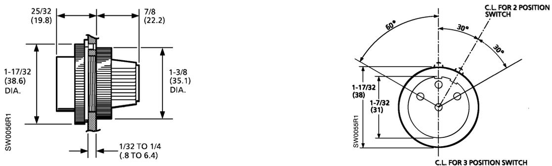
Figure 5. Dimensions of the SW 786 Selector Switches.
