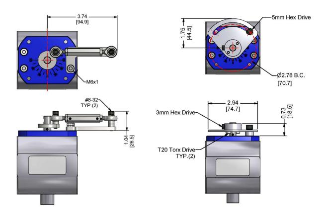
Figure 5: Dimensions of the AGA92.1 or VKG...-921 Manual Kit
