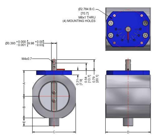
Figure 4: Dimensions of the VKG... Valve Shown on a VKG10.050U
