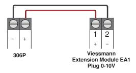
• Connect to the Viessmann Extension Module EA1 Plug 0-10V.
