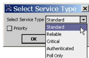
Selections “Standard, Reliable, Critical, Authenticated” set parameters per settings in the LonNetwork’s LonNetmgmt “Link Descriptors,” where timers are applied to the address table entry used for the link. Other parameters are applied to the Nv ConfigData on nvs (output side of the link).
