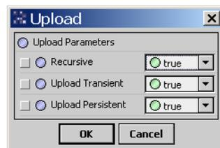
Typically, you leave dialog parameters at defaults (true)—recursive is always recommended. After using **Discover** and **Add** to create a new Lon device (and assigning the device a Lon Xml file), you can use **Upload** to populate current LonData in the device’s LonComponents (nvs, ncis, cps).
