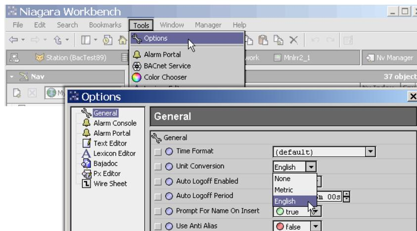
With Workbench unit conversion set to English, out values (for example, visible in a Lon device’s **Nv Manager** view, or within LonData in a device’s LonComponents) automatically display with the expected English units and corresponding numeric values. For related topics, see [“About the Nv Manager”](#) on page 3-31 and [“Using LonData directly”](#) on page 3-37.
