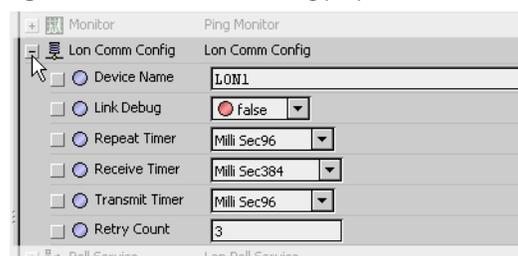
Typically, you leave all Lon Comm Config properties at default values, as shown in [Figure 3-8](#). The exception is when you have multiple LonNetworks (physical Lon ports), where each LonNetwork must have a unique Device Name (LON1, LON2, etc.).
