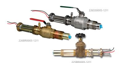
Insert-style hot tap liquid flow sensors with brass or stainless steel sleeves feature a ball or gate valve for pipe sizes 3" to 40" (77 to 1016 mm). These devices are designed for hot tap applications in pipes that cannot be drained for service. The HTT tool is required for hot tap installation. Use with a flow monitor or transmitter for a complete flow monitoring system.
