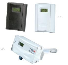
CDL/CWL carbon dioxide ( $\rm CO_2$ ) sensors maximize energy savings, while helping optimize ventilation. These sensors allow ventilation systems to be controlled by the amount of  $\rm CO_2$  present in a space. The CWL/CDL Series detect fluctuations in  $\rm CO_2$  levels and signal ventilation systems to provide an inlet of fresh air optimal for the space at a given time saving energy and increasing tenant comfort.
