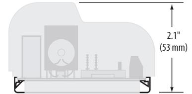
If the dust cover is ordered, the EP2 is mounted to a longer Snaptrack.
