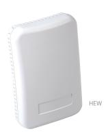
HEW Standard Series wall mount humidity transmitters offer high performance in an easy to install housing at an affordable price. The thin-film capacitive sensor element provides high accuracy and performance, great long-term stability, and full recovery from saturation. Temperature sensing options are also available.
