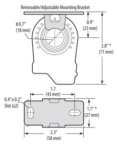
\* Terminal block may extend up to 1/8" over the height dimensions shown.
