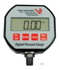
The versatile PD Digital Pressure Gauge can be used with any gas, liquid, or solid that is compatible with 17-4 stainless steel. The one-piece construction employs no silicone oil, welds, O-rings, or seals, making it the ideal universal pressure measurement device. The large LCD display shows the current reading, the selected scale, and the maximum and minimum pressure. All functions are easily controlled from the four panel push buttons located below the display.
