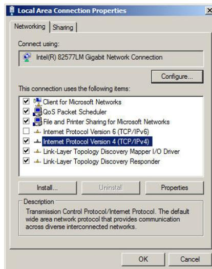
e. Select <Use the following IP Address>. Make note of the IP address that appears, then enter the static IP address (e.g. if the E8951 is still set to its default address of 192.168.1.24, then change it to 192.168.1.100). Enter 255.255.255.0 for the subnet mask. Click OK.
