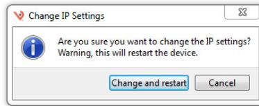
Confirm that the settings you entered are correct and click the Change and Restart button. The E8951 will reset and power up with the new settings. If you watch the Veris Toolbox screen, the entry for the old address will soon show a lost connection. Eventually a new entry with the new IP address will appear and the old entry will be deleted.
