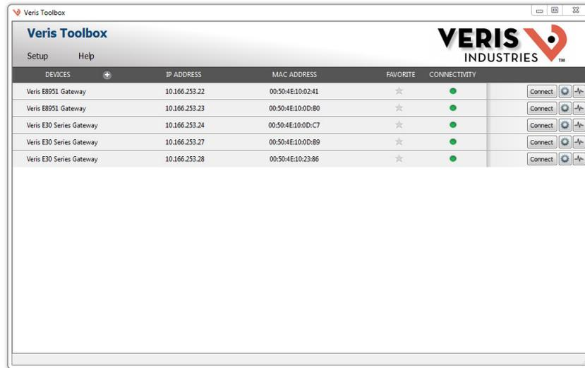
7. Click the gear-shaped configuration icon near the right edge of the window on the line that shows the device you wish to configure. The Configure Device dialog will appear.
