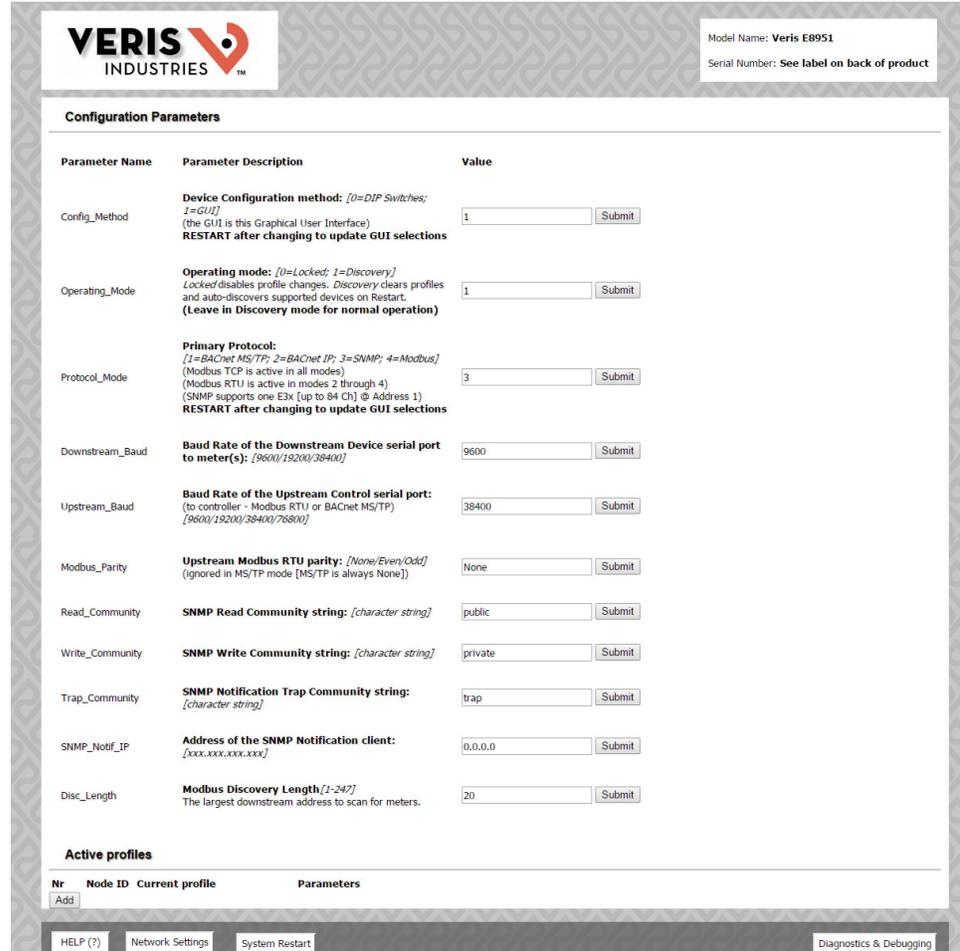
The screenshot shows the configuration web interface for a Veris Industries E8951 device. The page title is "Configuration Parameters". The interface includes a table of configuration parameters, each with a description and a value field with a "Submit" button. The parameters are:
