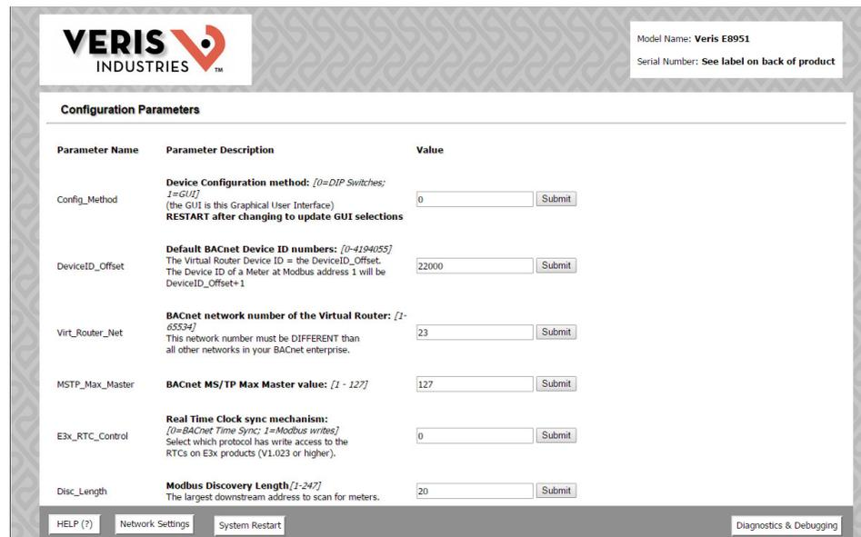
To set the IP address parameters, click the Network Settings button. The Network Settings overlay appears.
