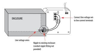
Wire the 12 AWG lines from the controller through the side of the device, from the enclosure to the line current terminals. Tighten line current terminal blocks to 12 in-lb (1.35 N-m) torque.
