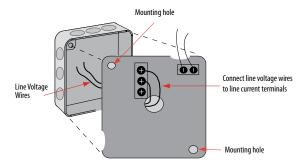
Wire the 12 AWG lines from the controller through the back of the device, to the line current terminals. Tighten line current terminal blocks to 12 in-lb (1.35 N-m) torque.
