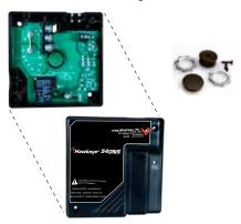
Wire the 24 AC/DC relay control through the top hole of the device. Use only copper conductors for command relay inputs. Tighten terminal blocks to 3.5 in-lb (0.4 N-m) torque. Keep wires away from the N. O. and N. C. jumper blocks.
