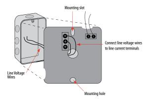
Wire the 12 AWG lines from the controller through the back of the device, to the line current terminals. Tighten line current terminal blocks to 12 in-lb (1.35 N-m) torque.
