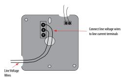
Wire the 12 AWG lines from the controller through the side of the device, onto the line current terminals. Tighten line current terminal blocks to 12 in-lb (1.35 N-m) torque.
