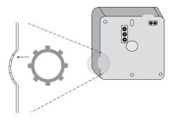
Insert the conduit nuts (provided) into the slots in the side hole of the device for additional weight support.
