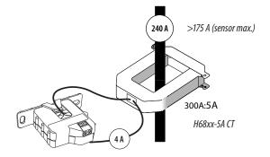
DANGER: 5A CTs can present hazardous voltages. Install CTs in accordance with manufacturer's instructions. Terminate the CT secondary before applying current.
