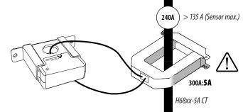
DANGER: 5A CTs can present hazardous voltages. Install CTs in accordance with manufacturer's instructions. Terminate the CT secondary before applying current.
