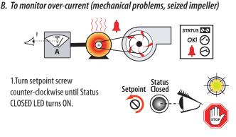
2. Slowly turn the setpoint screw clockwise until the Status OPEN LED just turns ON.
