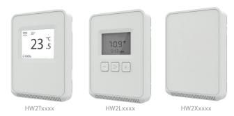
The HW2 Series of humidity sensors for living space is a flexible multisensor platform for use with BAS controllers designed to accept 4 to 20mA, 0 to 5Vdc or 0 to 10Vdc outputs. HW2 Series sensors are available with three user interface options: touchscreen, LCD with three buttons and blank. Humidity and temperature sensors are included with all HW2 Series sensors.
