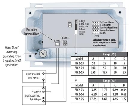
Optional: Connect Zero terminals to digital output (contact closure) of control system.
