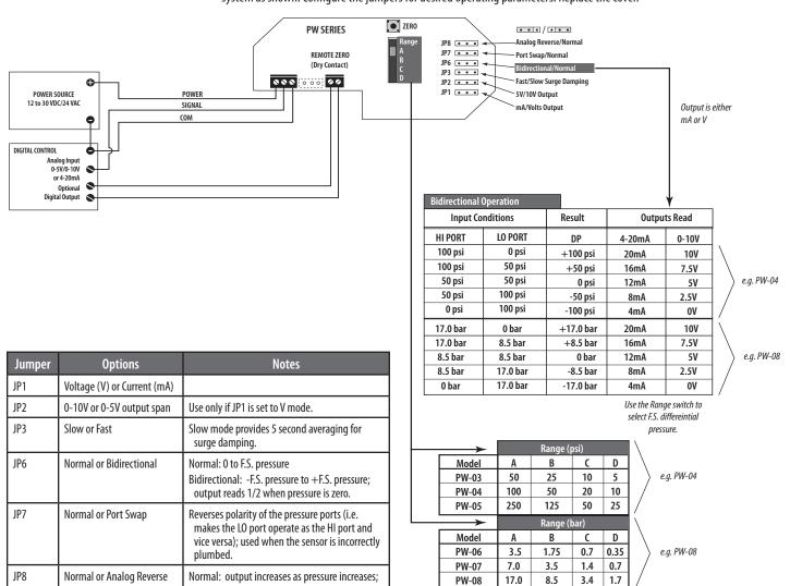
Reverse: output is maximum when pressure differential is zero and decreases as pressure
